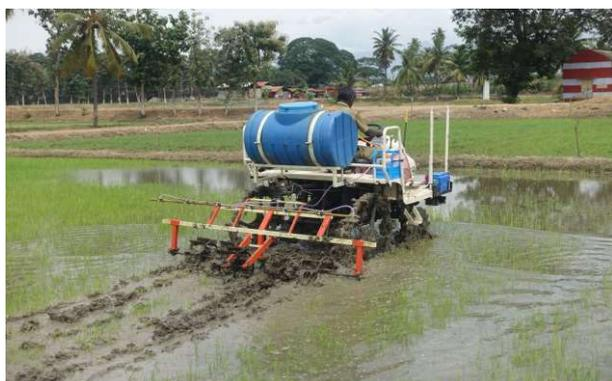
cum-sprayer can save 68 and 30% time as compared to weeding with power weeder and manual spraying with knapsack sprayer, respectively. The saving in cost of operation can be achieved by 96 and 93% as compared to weeding with power weeder and spraying with knapsack sprayer, respectively.
